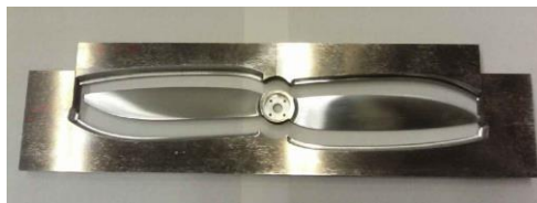
Fig.5 Profile cutting using WEDM
