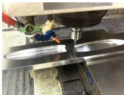
Fig.4 Direct endmilling using MC
